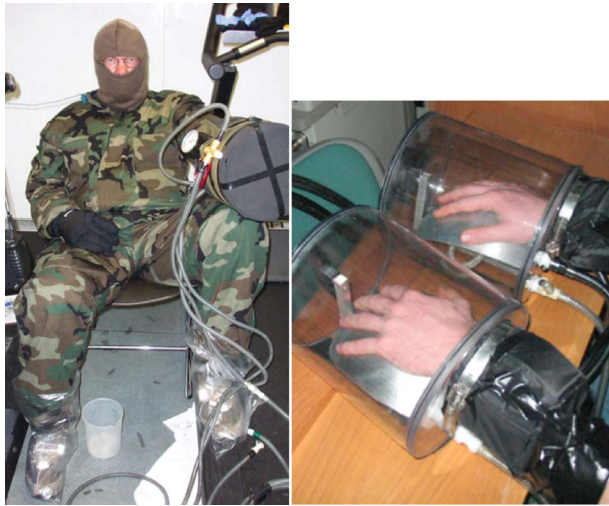
Fig. 1 Photographs of the experimental setup and experimental devices. Left panel: a subject clad in MOPP gear, balaclava, winter glove, and boot covers, and one hand in the experimental heat transfer device during postexercise rest in the experimental chamber ( T_{es}=41^{\circ}\text{C} ). Right panel: two hands placed in the experimental devices (see Sec. 2 for description of devices). The external neoprene insulation covering the experimental device had been removed for the photograph to better display the details of the device.
